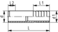
**SYGEF Standard Druckschlauchtülle SDR21/PN16**
